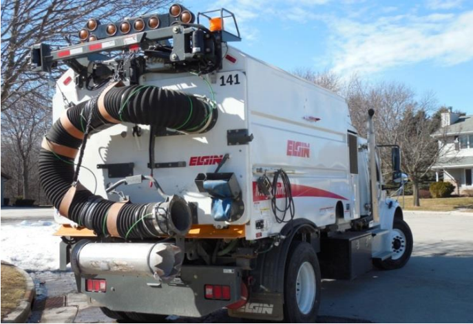
Sewer Whirlwind Catch Basin Cleaning Truck
